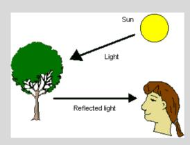
**Reflection** occurs when a light beam changes direction on hitting an object. The light bounces off the object at the same angle it hits it.
